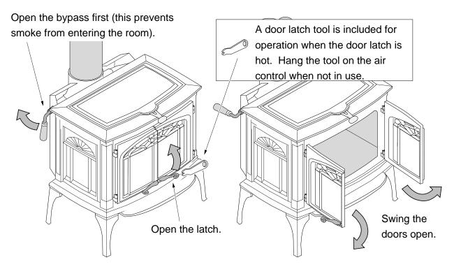
**WARNING**: Do not swing the doors past 90°. This may cause the doors to strike the body of the stove and cause damage.
